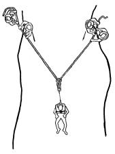
include a drill where I tether each student in the middle of the river and have them purposefully release from the jacket. This drill gives the student an idea of how an air pocket will start to form over the head of a trapped victim; and also how such a two point system could be used in a very high-risk application to lower a rescuer down to an entrapped victim. Again, the jacket doesn't always
