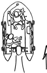
as far as possible, if necessary over the bow, helping to get the boat up on plane quickly. As soon as the boat is on plane, the deckhand moves back to the normal position.
