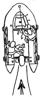
After a few seconds at full throttle, the coxswain calls, "stopping, now," the deckhand moves back as far as possible to the stern. As the coxswain comes off the throttle, the weight shift to the stern will cause the boat to "plow" to a halt. the stern partially submerging and dragging the boat to a stop virtually within its own length.
